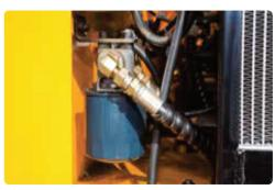
Remote Engine Oil Filter(HSL850-7A)
