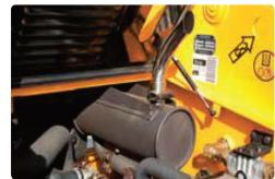
Frame Mounted Muffler reduce vibration and noise and improve durability.
