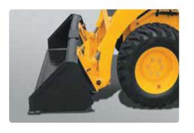
**Quick Attachment System** A quick attachment device improves cyc ease of operation.
